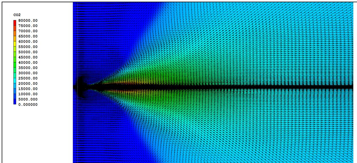
Figure 3: Velocity Field- Particular and vector field coloured by CO<sub>2</sub> ppm
