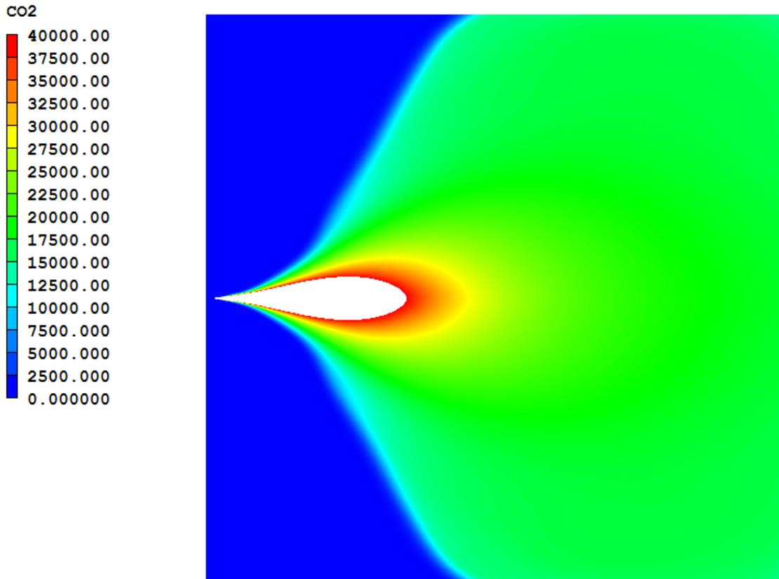
**Figure 7:** CO<sub>2</sub> concentration in ppm –Top view. The maximum ppm showing is set at 40000
