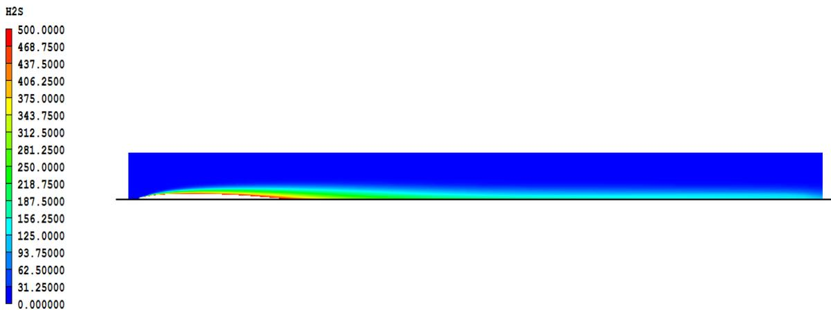
**Figure 8:** H<sub>2</sub>S concentration in ppm –Side view. The maximum ppm showing is set at 500
