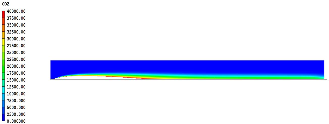
Figure 5: CO<sub>2</sub> concentration in ppm –Side view. The maximum ppm showing is set at 40000
