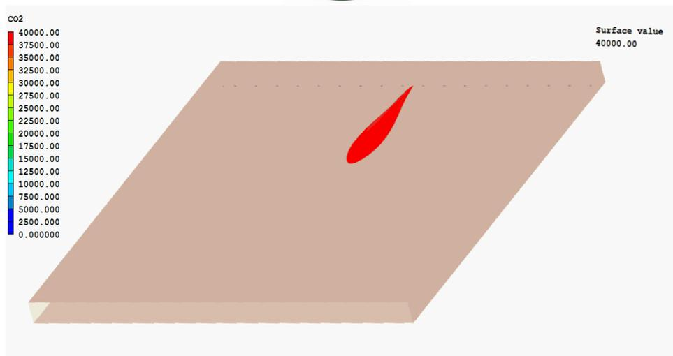
**Figure 11:** Iso-surface of  $\text{CO}_2$  concentration; 40000 ppm
