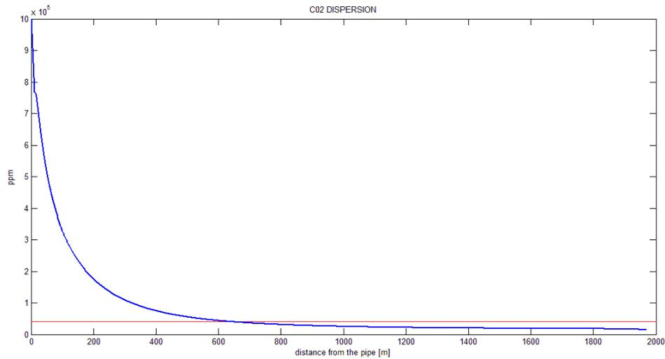
**Figure 16:** CO<sub>2</sub> dispersion in the y direction. In red the 40000 ppm concentration is highlighted
