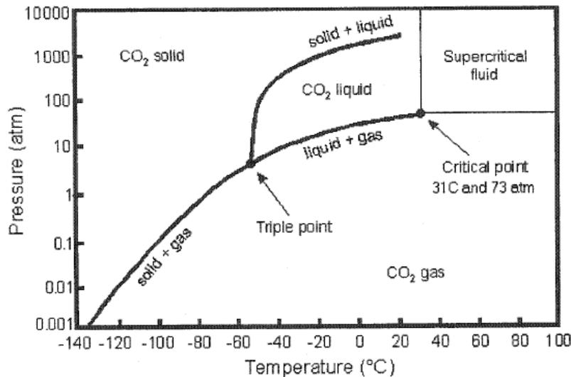
**Figure 1:** CO<sub>2</sub> phase diagram
