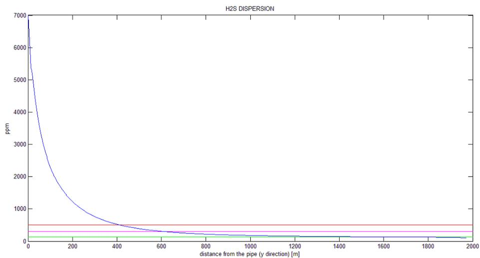
**Figure 17:** H<sub>2</sub>S dispersion in the y direction. The concentration at 500, 300 and 130 ppm are highlighted in red, magenta and green respectively
