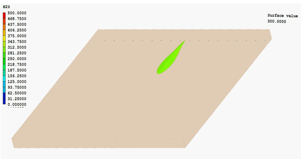
**Figure 13:** Iso-surface of  $\text{H}_2\text{S}$  concentration at 300 ppm
