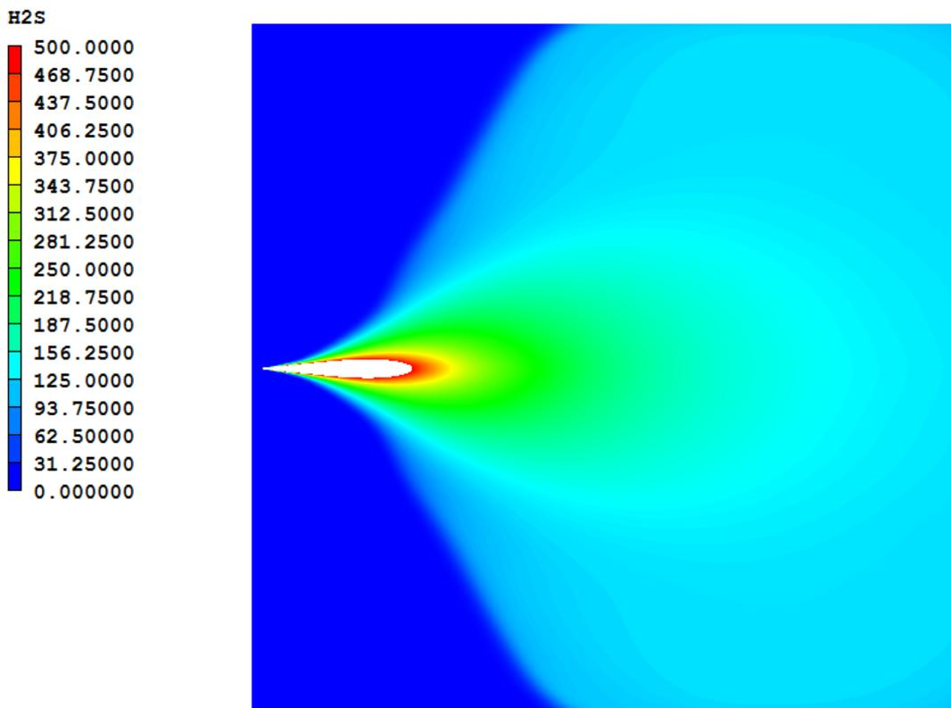
Figure 10:  $H_2S$  concentration in ppm- Top view. The maximum ppm showing is set at 500ppm
